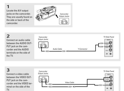
The audio-video cables shown here are usually included with a Camcorder. (If not, check your local electronics store.) If your camcorder is stereo, you need to connect a set of two cables.
